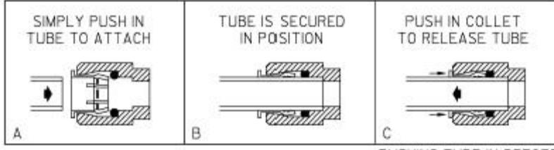
First, shut off the water supply. Cut a section of the tubing, enough to accommodate the filter. If your line has some flexibility, one cut may be enough. On copper tubing, be sure to remove any burrs. Attach the tubing to the inlet side. Slowly turn on the water supply, running the water into a bucket. This will flush the carbon fines from the filter. Shut off the water again and attach the outlet side. Turn on the water and check for leaks.
