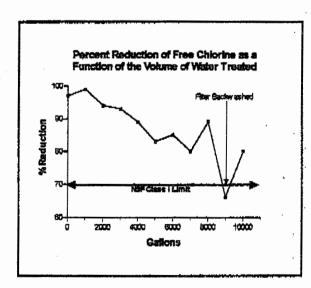
this instance 4000-gallons. However there was considerable iron fouling of the medium which lowered the filters performance. It is felt that with periodic backwashing of the filter it would remain 90% efficient for well over 8000-gallons.
