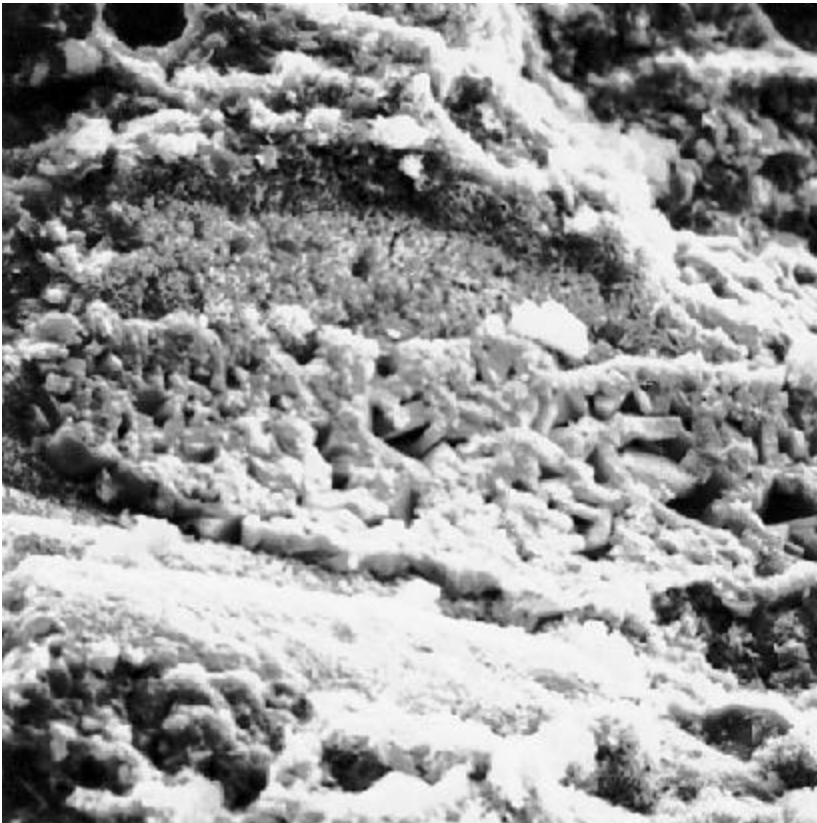
Figure 2. High magnification, photomicrograph of a sorbent granule surface. Note the intercrystalline structure & pore spaces (2 -10 microns) that provide high, surface area for water/liquid filtration of TSS particles. The granules provide ~8 fold higher “available filtration area than comparable sized sand/ anthracite beds.
